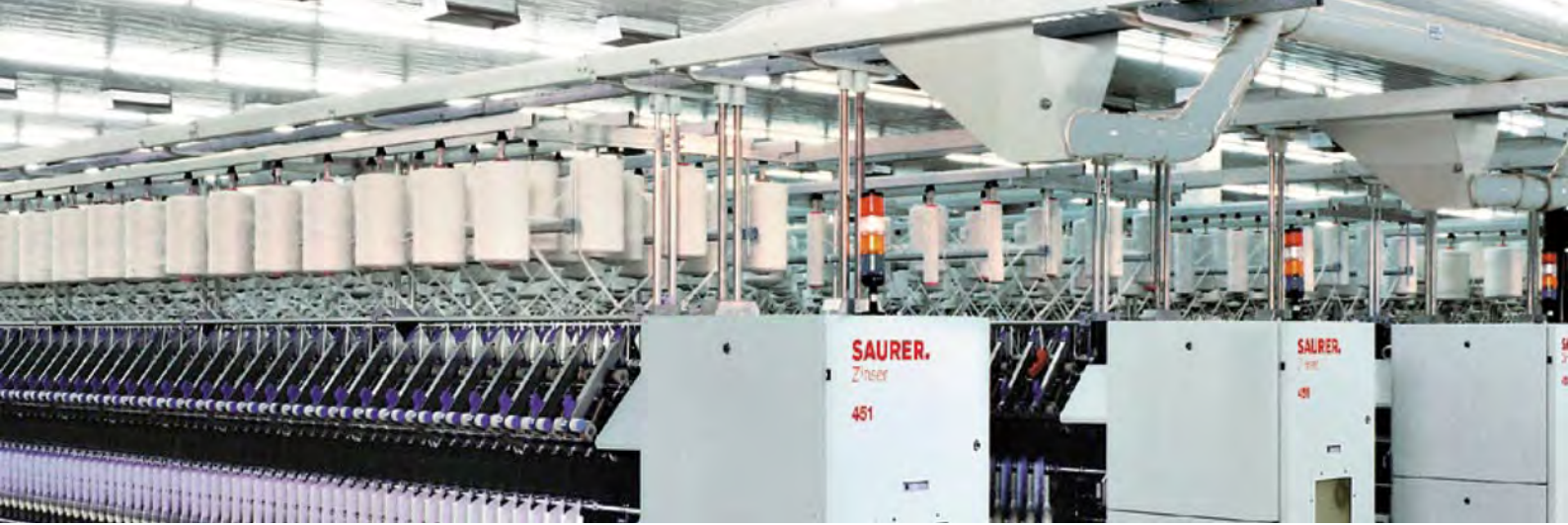
Autotex Bobbin Holder in Saurer Worsted Spinning Machine
