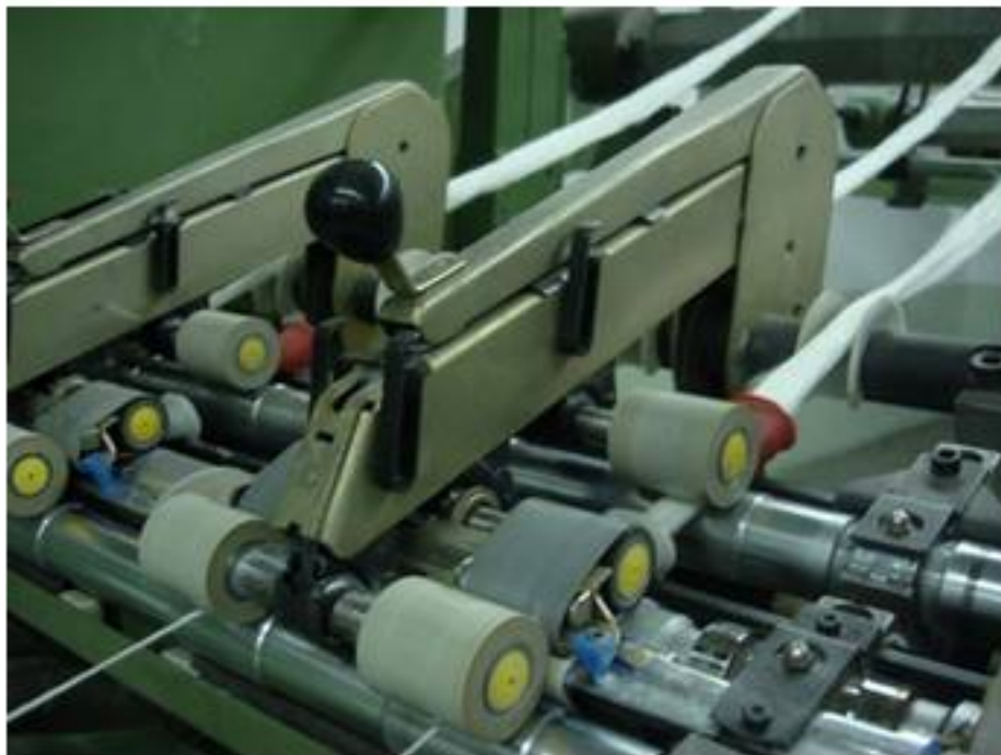
Fig: 3-over-3 double apron drafting system
